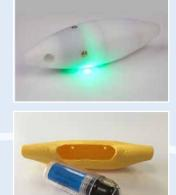
Examples of pingers: (top) a 70kHz pinger with an LED; (above) a Fishtek "banana pinger."
